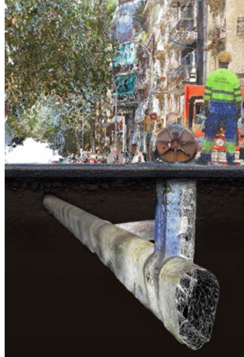
Actual 3D laser scan of a section of public road and an accessible sewer, represented as a point cloud.
